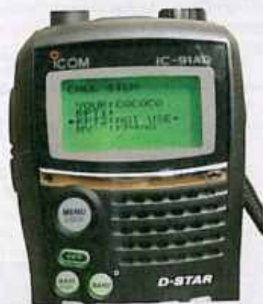
Figure 4 — Part of the extensive menu system on the IC-91AD handheld. It takes a minute to get used to what YOUR call sign and MY call sign mean. To talk to anyone, you program CQ in the YOUR field. If you wanted to talk to a specific station, you'd program that station's call sign in the YOUR field. If you want to use specific linked repeaters, you use the RPT1 and RPT2 fields. This is one radio you can't operate without some quality time in the manual.
