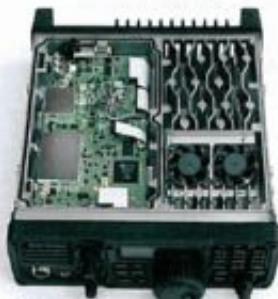
Opening the top cover reveals the main PCB and substantial fan-blown heatsink.
