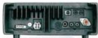
The USB port is a most welcome addition to the usual array of rear panel connectivity.
