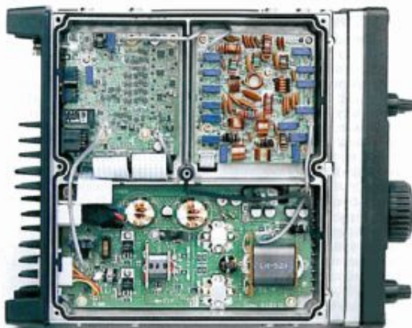
Underside the bottom cover are the PA board, output low pass filters and front end filters.
