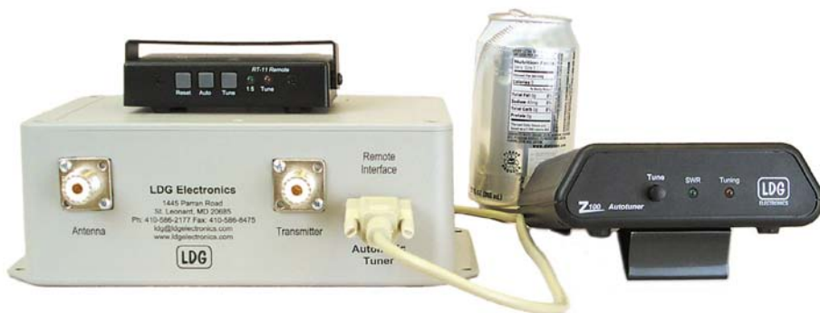
Figure 2—LDG RT-11 (left) with control box and Z-100. A 12 ounce beverage container is included for scale.
